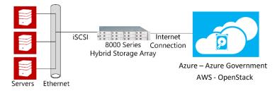
Figure 2. Network topology of 8000 series hybrid storage arrays
