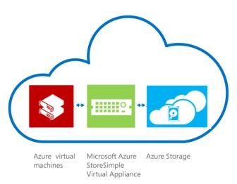
Figure 4. The Microsoft Azure StorSimple Virtual Appliance allows Azure VMs to access on-premises data uploaded by 8000 series hybrid storage arrays
