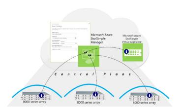
Figure 3. The Azure StorSimple Manager manages 8000 series arrays and a StorSimple Virtual Appliance over an Internet-connected control plane
