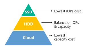
Figure 1. Storage tiers in a StorSimple 8000 series hybrid storage array
