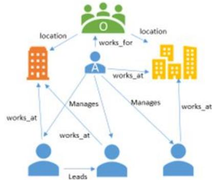
CRUD operations with SQL Graph effectively create nodes to represent various entities and create edges to represent relationships between any two nodes. Both nodes and edges can have properties associated with them. In addition, SQL Graph can perform multi-hop navigation in a graph using pattern matching (no joins). SQL language extensions for graph support enable join-free, pattern-matching queries for multi-hop navigation.
